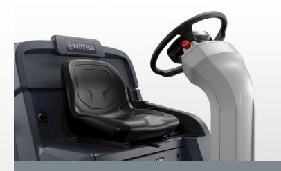
Ergonomic operator compartment with adjustable seat, steering wheelmounted controls, and speed paddles for frequently used functions.
