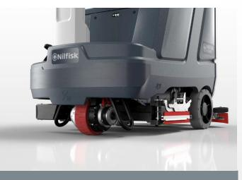
Compact design delivers superior maneuverability through aisles (minimum 1.6m width), high productivity with 140L tank capacity, and scrub-path width of up to 91 cm. Perfect for narrow aisles becoming more common in warehousing.
