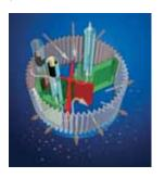
The XtremeClean technology\* is based on a valve controlled principle, using the air flow to clean one half of the filter cartridge - despite still work- ing with the other half. The dirt is blasted off the filter and the suction performance is always maintained.
