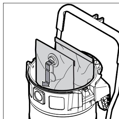
4. Insert the filter bag (C) in the dirt tank.
