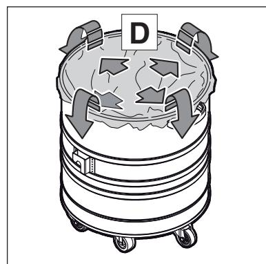
5. Insert the disposal bag (D) in the dirt tank.
