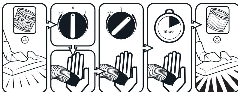
To ensure that suction performance is always at its best, the filter element is automatically cleaned during operation. We recommend complete cleaning if the filter element becomes extremely dirty.
