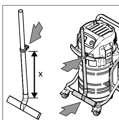
1. Attach the suction pipe holder to the suction pipe.
