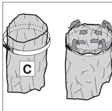
4. Insert disposal bag (C) into clamping ring.
