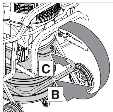
7. Push the dirt tank as far as possible into the vacuum cleaner.
