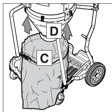
6. Attach the new disposal bag (C) onto the storage container (D).
