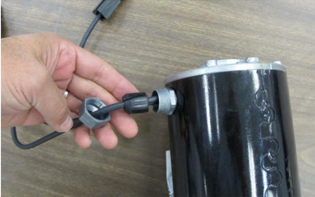
3. Mark orientation of end plates to motor housing and remove both through bolts.
