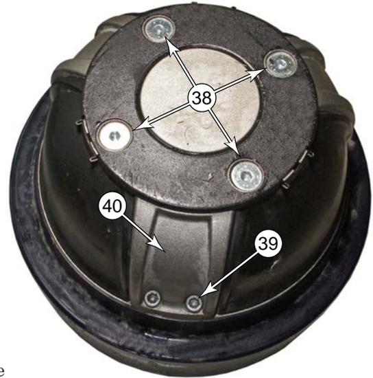
For reference, the wheel/tire presses over the main bearing (42). The drive hub (40) is lightly pressed onto the tapered disk (43) of the gearbox.
