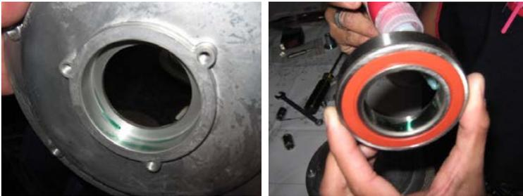
2. Press the bearing into the driver motor.
